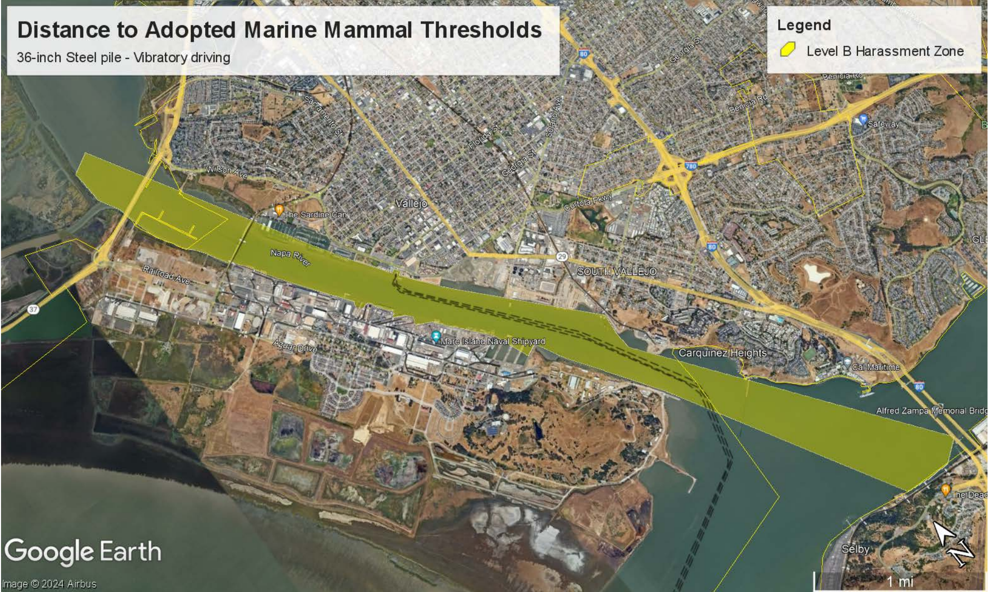
FIGURE A6 Distance to Marine Mammal Thresholds for 36-inch steel piles using vibratory hammer (Google Earth 2024)
