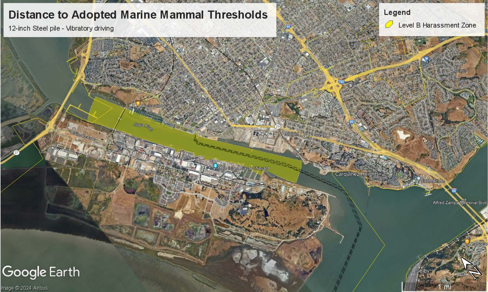
FIGURE A4 Distance to Marine Mammal Thresholds for 12-inch steel piles using vibratory hammer (Google Earth 2024)
