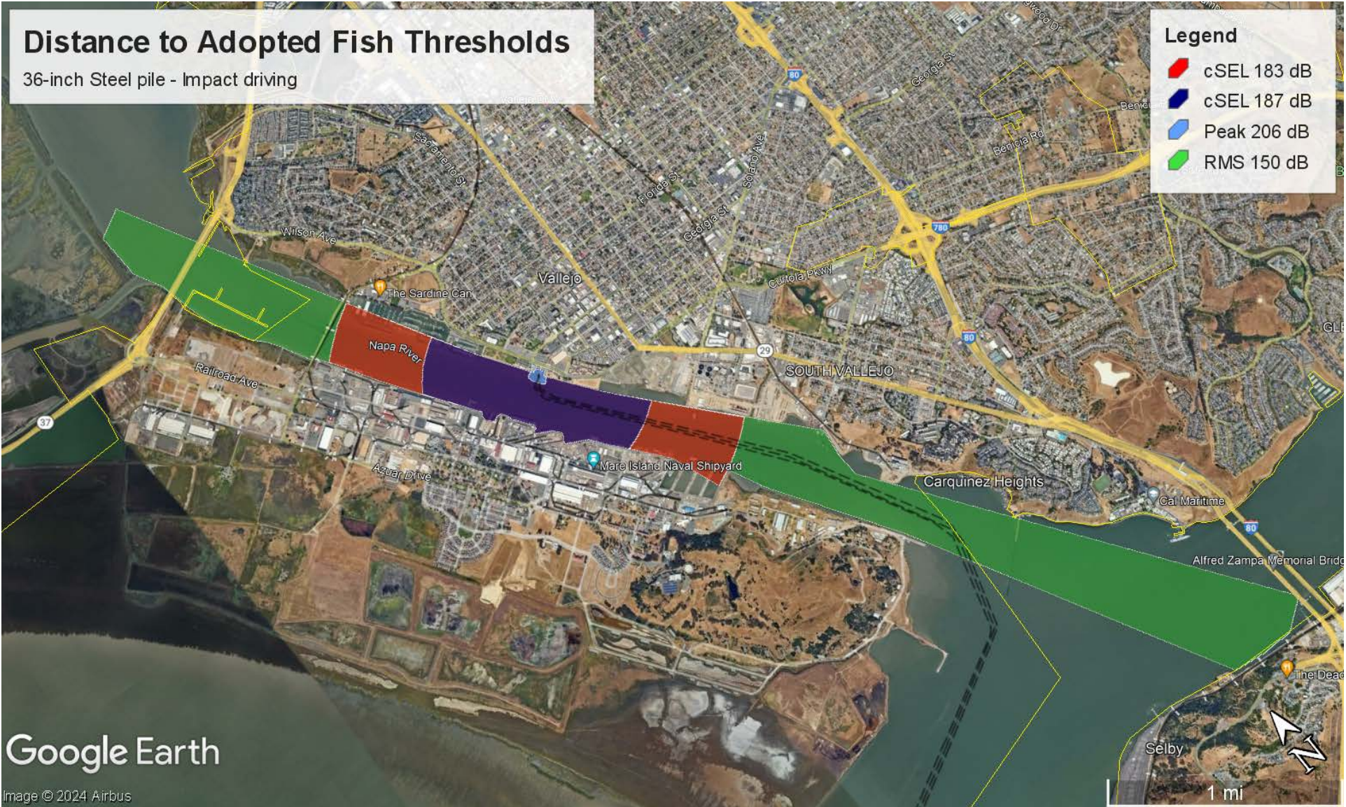
FIGURE A2 Distance to Adopted Fish Thresholds for Unattenuated 36-inch steel piles impact driven (Google Earth 2024)
