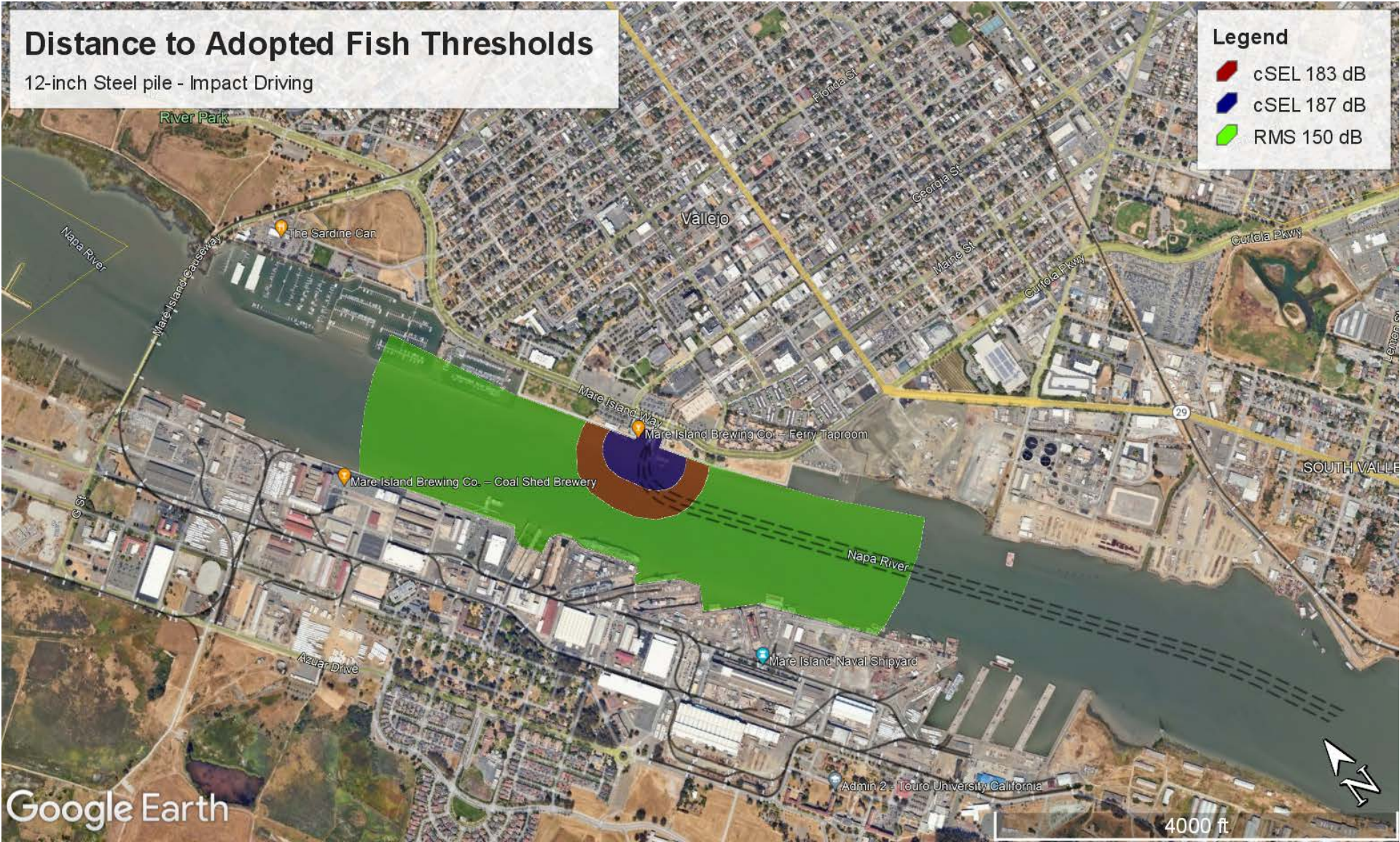
FIGURE A1 Distance to Adopted Fish Thresholds for Unattenuated 12-inch steel piles impact driven (Google Earth 2024)
